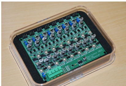
Figure 6: ESCHER-MIC8 8 channel condenser pre-amplifier
