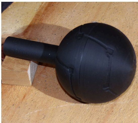
Figure 9: MEMSAAMA 3D-Printed Ambisonics microphone case, first version
