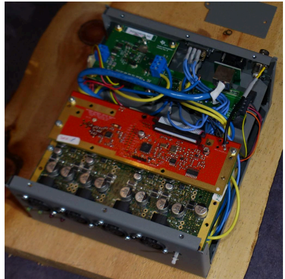
Figure 3: WILMA box with charger, battery, pre-amplifier ...
