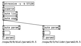
Figure 1: Pd patch with two OSPW parameters.
